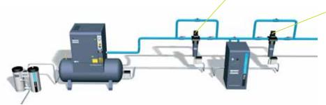
The final filter will remove particles to 0.01 micron and oil to 0.01mg/m<sup>3</sup>.
